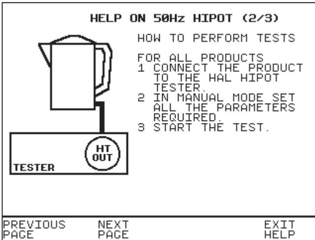
A description of how to connect the test leads and perform the test is provided in a step-by-step format.
