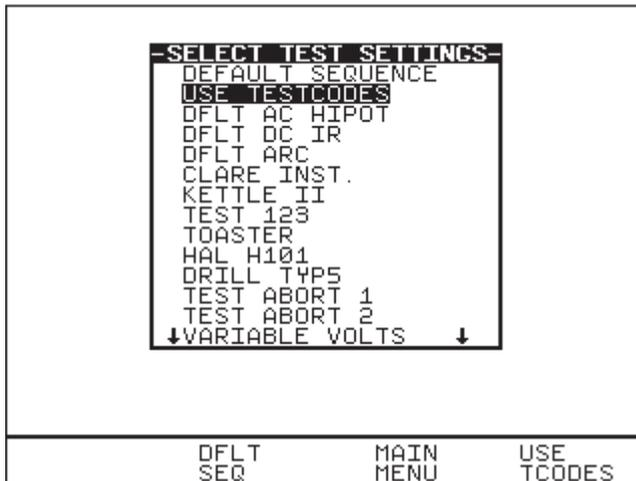
Use the encoder to highlight a Test Sequence Setting and press the green button to select the desired option.
