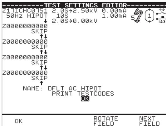
Use the encoder to highlight a field to be changed and press Green to select the desired option. Use the fast key to highlight the desired field, and the encoder to cycle through the range of permissible values for the test parameter. Use the fast key to enter the value. To exit this editing phase, select the OK fast key. Changes will be stored to the system. These fields have been described in detail under the Default Test Settings section.
