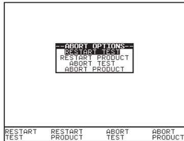
Use fast key functions or the encoder to highlight an action following abort and press the green button to select the desired option.
