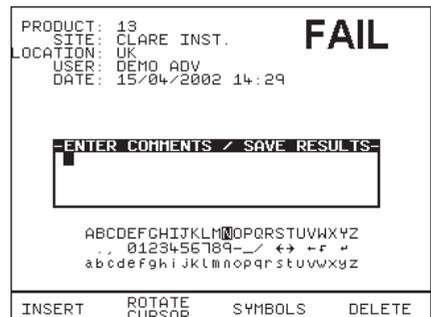
Fail Comments – Use encoder & Insert key to enter in any comments. To skip line or move to next line, highlight Rotate Cursor and turn encoder. Or use barcodes.
