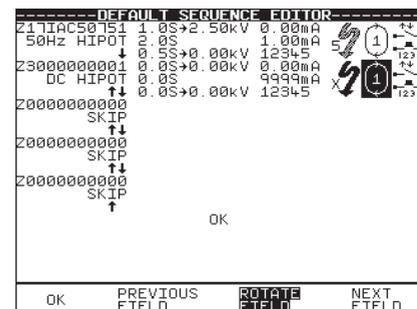
Caution: It must be noted that only the integer(s) selected will conduct the test voltage(s), a blank ' - ' will be by-passed.
