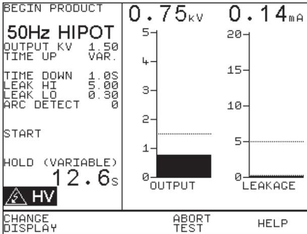
The screen can be considered as two panels, left and right. In the left panel the information is from top to bottom, as follows:
