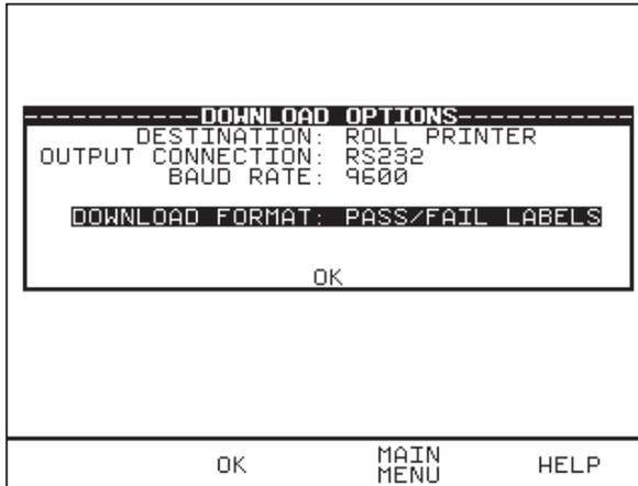
Use the encoder to highlight the required parameters. Use repeated presses of the green button to show the desired options for destination, output connection and baud rate.
